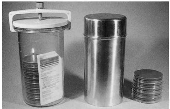
Plate 7.5 Systems for culturing in carbon dioxide. The jar can be used with chemicals which provide a carbon dioxide (CO 2 ) enriched atmosphere and the tin with a candle to provide CO 2 conditions (see text). Reproduced from Laboratory diagnosis of sexually transmitted diseases , WHO 1999, with the permission of the World Health Organization.
